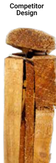
Capping rail 'popping off'
