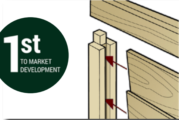
Rebated frame and Mortise and Tenon joint
